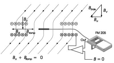
Figure 2 Compensation of an external magnetic field
